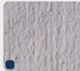
CSP-4 LIGHT SHOT BLASTING
