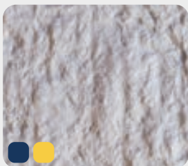
CSP-6 MEDIUM/HEAVY SHOT BLASTING OR LIGHT SCARIFYING
